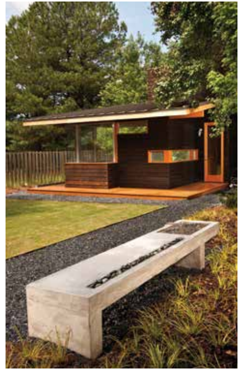
OPPOSITE: THE BENCH WAS MADE IN ONE PIECE USING GLASS-FIBER-REINFORCED CONCRETE. NO PIGMENT OR SPECIAL FINISHES WERE ADDED. ABOVE LEFT TO RIGHT: THE WATERFALL, GENERATED BY A RECIRCULATING PUMP, FLOWS OVER THE EDGE IN A GENTLE CASCADE; A FURROW IN THE BACK OF THE BENCH CHANNELS THE WATER OVER A BED OF NATIVE RIVER ROCK; COMBINING THE ORGANIC ELEMENTS OF CONCRETE, STONE, AND WATER, THIS WABI-SABI STYLE GARDEN BENCH IS THE IDEAL SPOT FOR REFLECTION AND MEDIATION.
