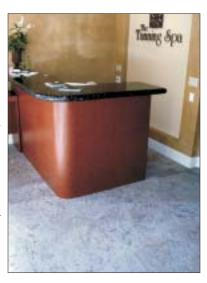
These self-leveling overlays are flowable, polymer-modified cementitious toppings that have the huge advantage of setting within a matter of hours, says Bruce Hackett of Concrete Décor magazine.
